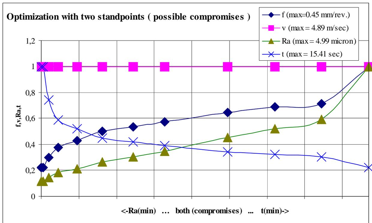
Figure 5. Parameters resulted by the optimisation of the plate turning operation. On the left side the viewpoint of the customer ( $R_a$  - min.) on the right side the viewpoint of the producer ( $t$  - min.) is satisfied. Curves show possible compromises between the two viewpoints.
