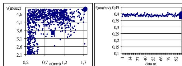
Fig. 3. A thousand of possible machine settings are presented as small rhombuses in the pictures to produce the surface with the given roughness. Circles in the pictures represent the original machine setting. Large squares represent estimation of the classical method.
