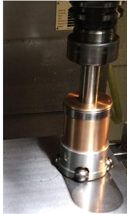
Fig. 11. The permanent MABB tool during machining
