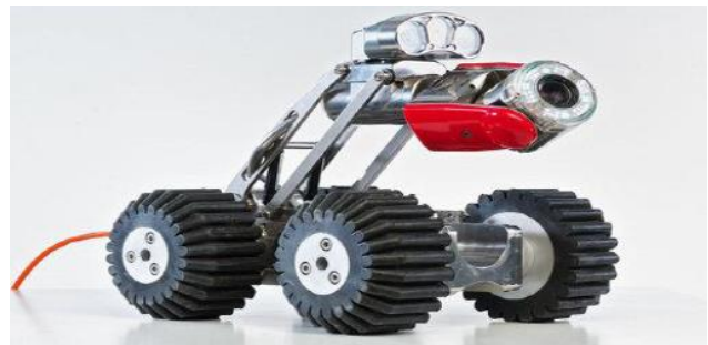
Fig. 1. Remotely controlled CCTV camera used in drain and sewer systems inspections [8].
