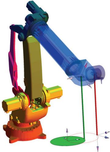
Fig. 5. Closed-form solution for a kinematic chain without offset (green beam), and one-dimensional iterative search for the real TCP (red beam).
