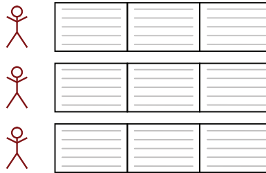
Figure 1: A warehouse operated by 3 pickers, with 3 zones for each picker. Physically, each zone is composed of a matrix structure of aisles and cross-aisles.
