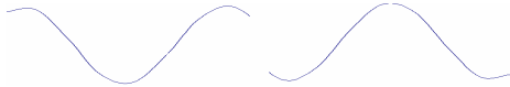
Figure 4. Illustration of shapes of image row functions where possibly a vertical scratch goes through (left: darker, right: lighter).
