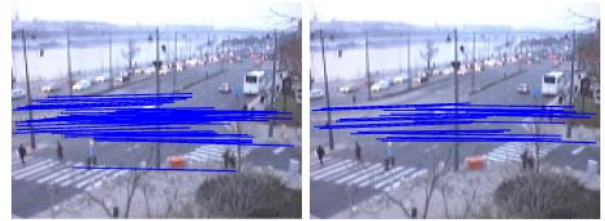
Figure 2 Inliers for the real-valued motion history vectors and on-line entropy based feature extraction (left image); and for the binary motion history vectors and on-line entropy based feature extraction (right image).
