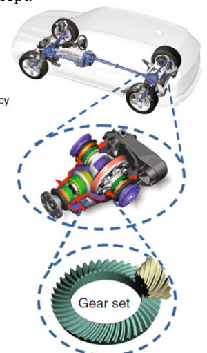
Figure 4. List of requirements on the Hypoid gear sets for passenger vehicle axle drives of standard design.
