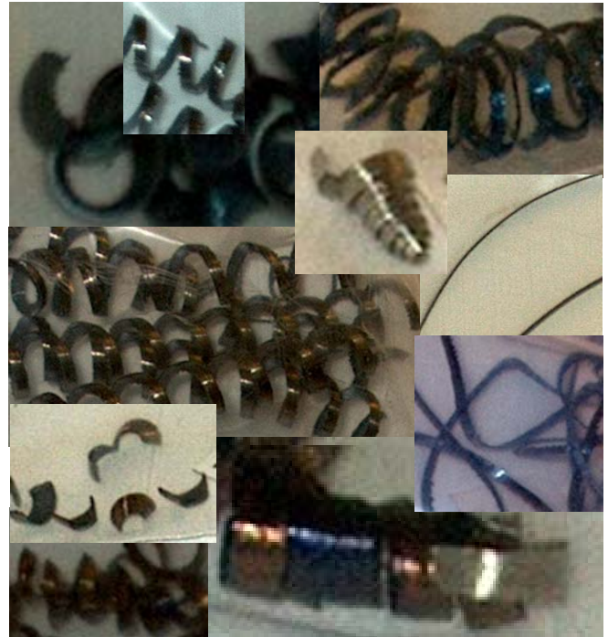
Fig. 3. Some collected chips, showing the variety in their forms
