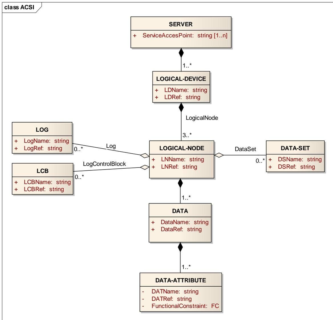
Fig 3: Conceptual class model of the ACSI
