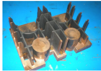
Figure 2: A complex die-sink EDM electrode causes a high manufacturing cost.
